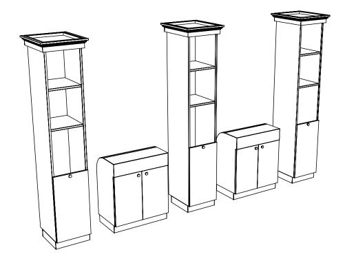
Adjacent cabinets and components should be assembled by fastening through the interior panels with the screws or bolts provided. Tighten securely.
